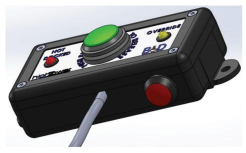
When pressed, the override sends a signal to the HighTower Docking Station that cancels out both the audible and visual alarm that sound when the HighTower senses ignition but not a docked power wheelchair. This is especially useful when the vehicle will be operated but the HighTower Docking Station will not.
